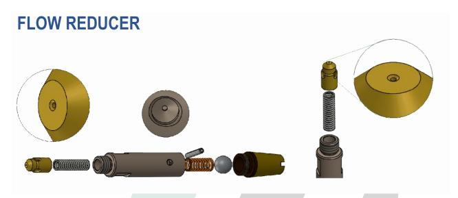
8 The flow regulator is integrated into the valve body, its function is to open fully during cylinder filling and to narrow the passage, via a pre-calibrated hole. during outlet refilling.
